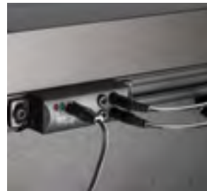
IR Repeater allows remote controls to operate through solid doors
