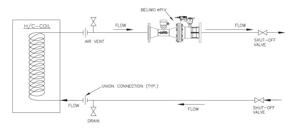
Electronic Pressure Independent Valves can be piped in a parallel orientation to achieve increased flow rates.
