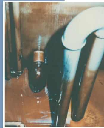
Oxidation in oil reservoir – curable with Kleentek
