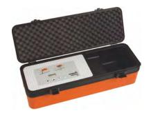
As an **alternative** to the **G 100** signal generator, with 10 W transmitting power, the more powerful **G1** generator with up to 50 W transmitting power can be used. There are various accessories available for this generator.
