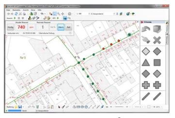
This screenshot shows the SeCuRi® SAT Complete user screen. The control panel for the gas leak detector is in the top left corner.
