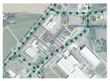
This screenshot shows a pipe network plan set against an aerial view (grid data). Red and green dots mark the inspected route. Red dots indicate a leak which has not yet been located and classified. Yellow Xs are inspected house service connections, red Xs are house service connections which have not been inspected.
