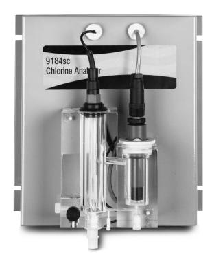
The low minimum detection limit and wide measurement range of the Hach 9184 sc Amperometric Free Chlorine Sensor makes it ideal for efficient residual chlorine monitoring. Continuously measure hypochlorous (HOCI), temperature, and pH. WW
