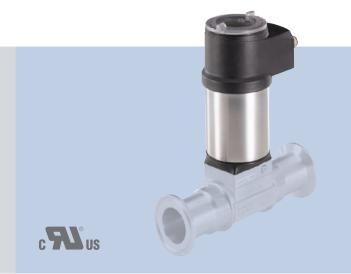
Unique bayonet style flow meter constructed from an SE36 sensor and any of the S030 fittings shown on page 65. This two-wire 4-20 mA INLINE flow meter is manufactured to provide true, reliable flow for neutral, solid free liquids. A backlit removable display makes the system adds more value as it can program multiple transmitters.
