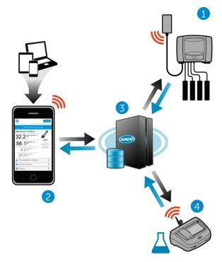
The communication between the Hach instruments seen in (1) and (4) is established through Wi-Fi or a 3G/4G modem.
