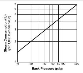
Capacity of GT14M as a steam trap (P1 > P2). Instantaneous condensate loads above the rated trap capacity will cause the pump to cycle and therefore reduce the discharge capacity.
