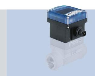
Unique bayonet style flow meter constructed from an SE32 transmitter and an S030 flow fitting. A large digital display with 3 button keypad and bargraph make this perfect for neutral, solid free liquids. Hysteresis and goalpost switching make this an intelligent component in any flow control loop.
