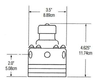
The topworks of the valve must have six,  $1/4-20 \times 9/16$  deep holes (minimum) blind tapped, equally spaced on a 03,000 B.C. for mounting positioners.
