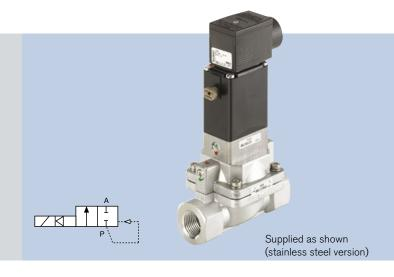
Completely unique servo-assisted solenoid valve with isolated pivoted armature pilot. This valve design is much less sensitive to fluid contamination than plunger operated valves and therefore offers many advantages in the process environment. The pilot section can be rotated in the field to make the valve Normally Open.
