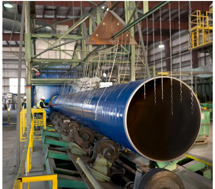
Polyurethane coating meeting the requirements of ANSI/AWWA C222 is available from AMERICAN. Polyurethane coating is typically applied at 25 mils minimum DFT, but thicker coating is possible. Contact an AMERICAN representative regarding increased coating thickness. The coating is applied and tested for conformance as described previously for polyurethane lining.
