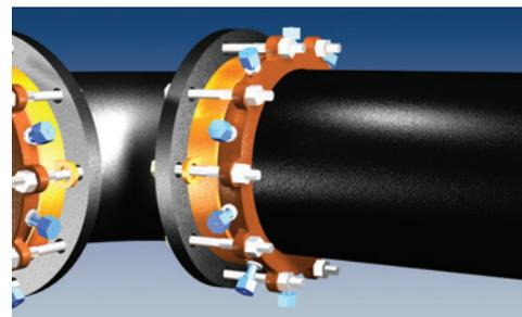
7. Tighten the actuating screws in an alternating manner until all wedges touch the pipe. Continue tightening the nuts in an alternating pattern until all the torque-limiting nuts have been twisted off.
