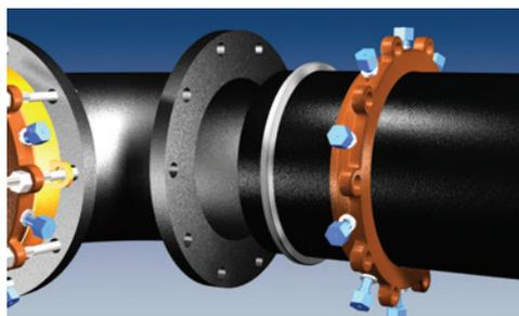
3. Lubricate and place the EBAA-Seal™ Gasket on the clean pipe following the restraint ring. (USE A TRANSITION GASKET IN PLACE OF THE EBAA-SEAL GASKET FOR STEEL AND IPS. O.D. PVC PIPE.)
