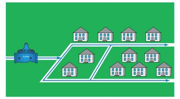
The CTC-33 Timer Control is used for pressure management applications in water distribution systems where SCADA control is not available. Use a 139 Series Cla-Val Pressure Control Valve equipped with the CTC-33 Timer to change pressure during periods of high and low demand according to pre-set schedule to reduce leaks and pipe burst frequency, while delivering adequate supply.
