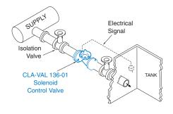
Liquid level control can be provided by using a float switch or electrode probe which sends an electrical signal to open or close the valve as needed.
