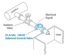
Industrial uses for the solenoid control valve are many and include accurate control of process water for batching, mixing, washing, blending or other on-off type uses.
