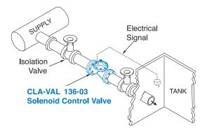
Liquid level control can be provided by using a float switch or electrode probe which sends an electrical signal to open or close the valve as needed.
