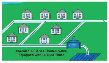
The CTC-33 Electronic Timer Control is used in 139 Series Control Valves to automate circulating water requirements in distribution system applications. Valve opening and closing time of day and duration can be set according to system requirements for convenient flushing and circulating during times of low flow to optimize water quality.
