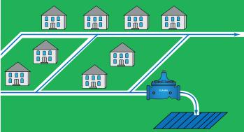
The CTC-33 Electronic Timer Control is used in 139 Series Control Valves to automate circulating water requirements in distribution system applications. Valve opening and closing time of day and duration can be set according to system requirements for convenient flushing and circulating during times of low flow to optimize water quality.
