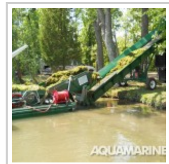
Aquatic transporter with feed through storage conveyor unloading system (bow to stern).
