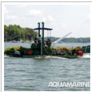
Aquatic transporter with feed through storage conveyor unloading system (bow to stern).
