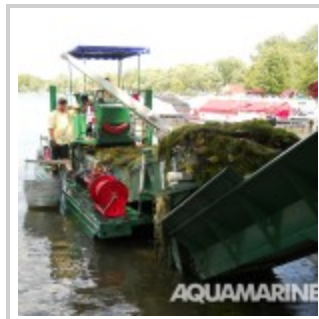
Aquatic transporter with feed through storage conveyor unloading system (bow to stern).
