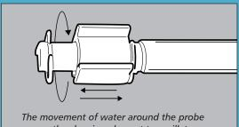
causes the cleaning element to oscillate, constantly removing lime build-up.
