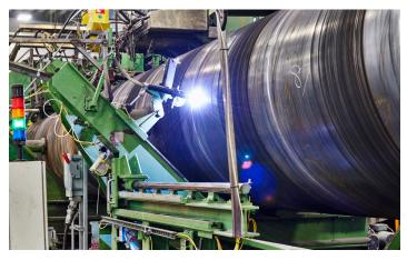
AMERICAN's spiral mills have the capacity to handle coils of steel from 0.1875 inches (4.8 mm) to 1 inch (25.4 mm) in thickness, with yield strengths up to 70,000 psi (482 MPa), to produce high-quality, spiral-welded steel pipe up to 144 inches (3,600 mm) in diameter. This flexibility offers AMERICAN's customers a wide variety of options.
