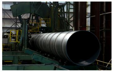
Finished pipe cylinders are moved through the production process by an efficient and ergonomically-friendly pipe handling system.
