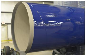
The polyurethane area includes two parallel pipe translators, or conveyors. The first set of translators move the pipe through a pre-heating cabinet to eliminate any moisture on the pipe and elevate the temperature of the pipe for application of the polyurethane. Immediately after the pipe exits the pre-heating cabinet, the pipe enters the blast cabinet where the surface is prepared for the application process.
