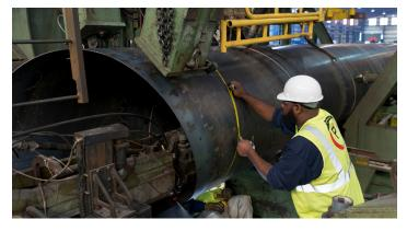
Pipe forming begins when the coils are loaded into the forming section. The steel coil is unwound and fed through the first of four sets of flattening rolls. The flattened coil continues through the forming section that is set at the required angle, based on the diameter of the finished cylinder, and the coil thickness and width.
