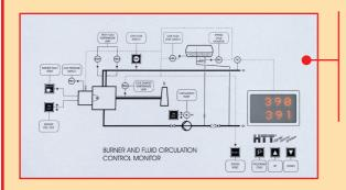
Powerhouse's integrated control panel monitors all gas and heating functions for immediate identification of process status; independent burner control buttons automatically synchronize the burner system with the ironer's actual production rate for highest efficiency and capacity. The easy to read status indicators and fault monitors make servicing simpler.
