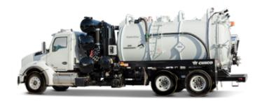
Your toughest jobs just got easier with Cusco's Turbovac truck series. Built to perform, Cusco's Turbovac series will handle heavy sludge, slurries, and liquid waste without compromise. With cyclonic filtration technology, airflow ratings of 1,800 CFM to 5,500 CFM, and powered with 28" Hg of vacuum, the Turbovac series is your solution to handling hazardous and non-hazardous waste removal and environmental remediation.
