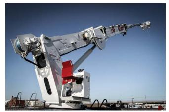
Boom trucks can also be customized with a 'Command Post' seated control station that rotates 360 degrees with the boom to provide optimized visibility and operator comfort.
