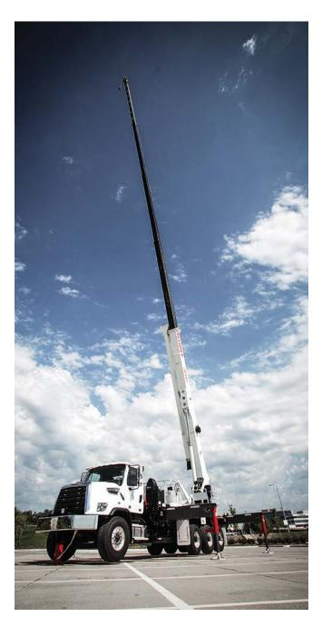
If your job calls for just a bit longer reach than what the powered boom can achieve, you can add an additional manual swing around section, or jib.
