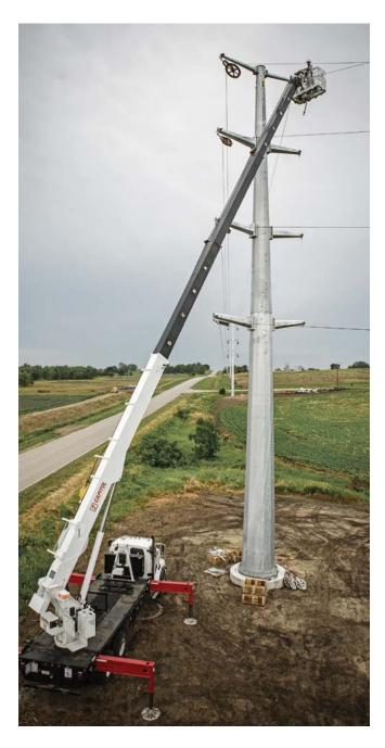
Boom trucks can be optionally equipped with work platforms that enable them to position people1 in addition to lifting loads. With an Elliott boom truck, work platforms come standard with a two-person detachable gravity-leveled steel basket with a hydraulic lifting system. Range diagrams and load charts can be found inside the basket for quick reference.
