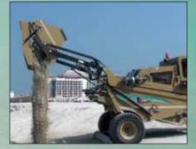
The Model 5500's clam-style hopper can be dumped to the ground or lifted to 102" (2600mm) for unloading into trucks.
