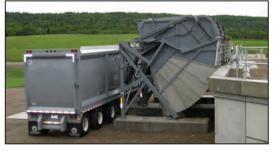
Integrates with walking floors and compaction trailers.
