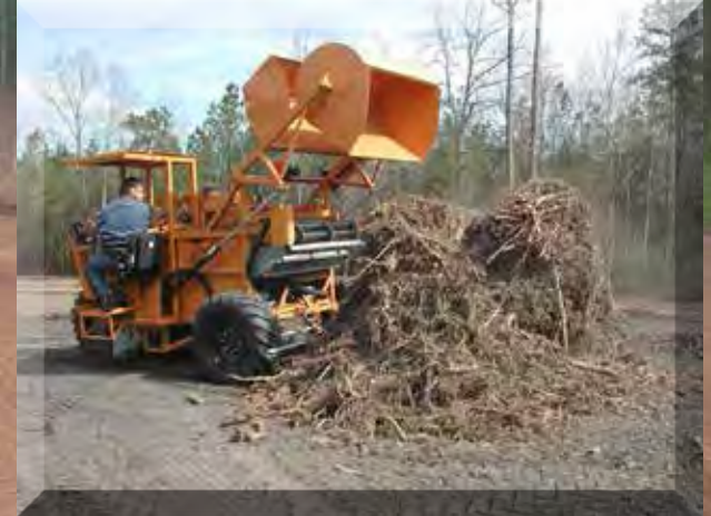
Remove roots and sticks up to 36 inches (914mm) long
