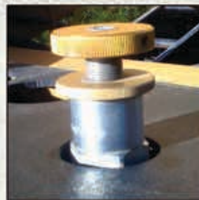
Oscillation control valve - select the exact amount of screen oscillation for varying conditions
