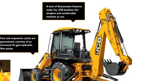
18,000lbs of swing torque, and 2" thick swing frame ensure robust strength when operating laterally.
