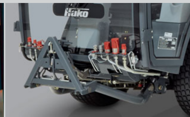
Fast, easy, no tools needed: thanks to the quick-change system, the Citymaster can be re-tooled for the next job in no time at all.
