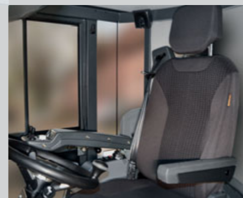
For even more efficient work results: driver's cabin with ergonomic comfort seats and one-hand operating system integrated in the armrest.
