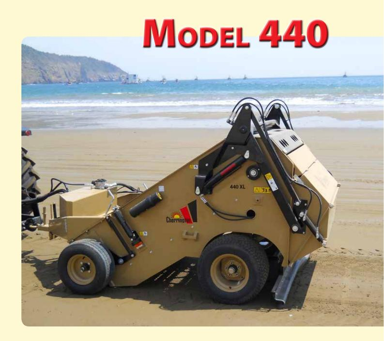
Cherrington lifts and screens the sand to screen-clean and sanitize your beach. Efficient and economical Beachcleaning using Cherrington Beach Cleaners is accomplished by lifting the sand from the beach, screening it through a powered oscillating screen, retaining all objects larger than the chosen screen size and then returning the sand to the beach.
