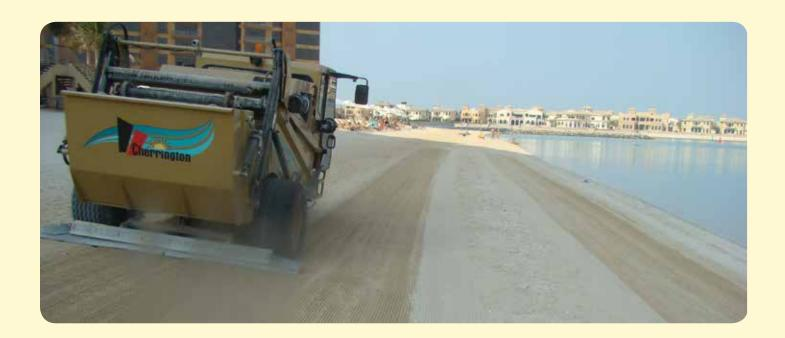
Cherrington's sifting screen uses a high speed hydraulic elliptical motor to produce a short, but intense, movement to the screen.
