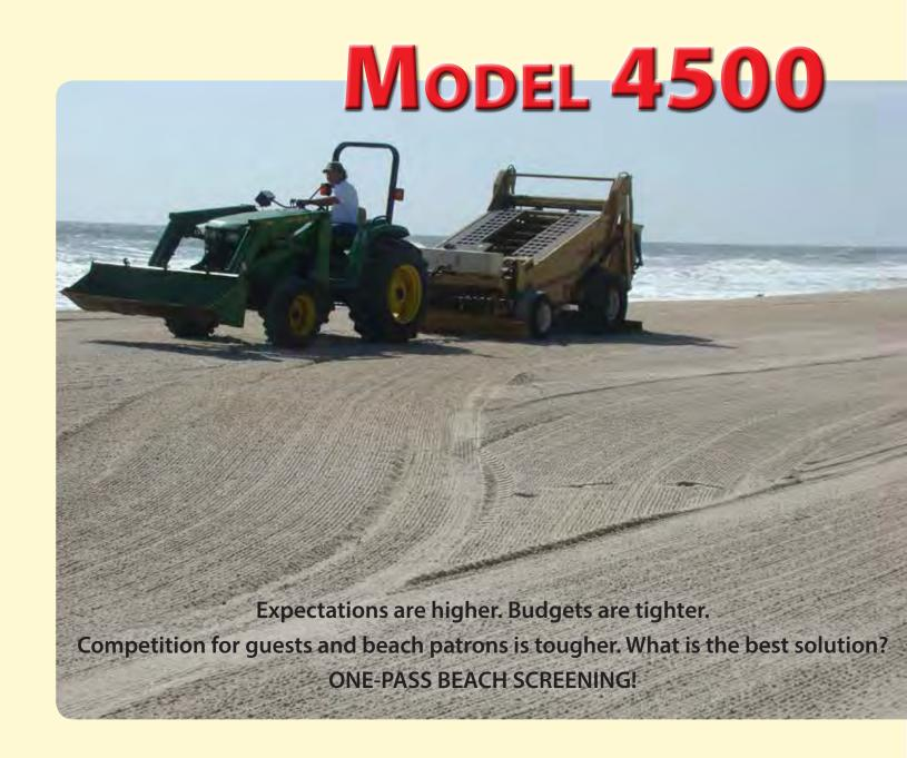
The Cherrington 4500XL is fast, rugged and dependable with only 3 bearings and no revolving belts, tines, or screens for amazingly low maintenance and long life. Carbide glide pucks for long life and smooth, quiet operation. Compact size and "power-delivered-to-the-screen" design.
