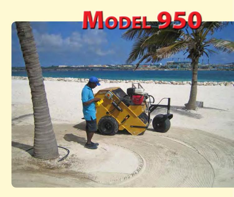
Like all Cherrington Screeners, the Model 950 efficiently collects everything larger than the selected screen-hole size. The Cherrington Model 950 is shipped with two separate interchangeable screens to allow you to adapt quickly to changing screening conditions. The  $\frac{1}{2}$ " (13mm) and  $\frac{3}{4}$ " (19mm) wire screens are standard and the  $\frac{3}{8}$ " (9mm) and 1 inch (25mm) screens are available for special screening needs.
