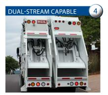
Dual-bin design allows for collection of trash and recyclables or two different waste streams.
