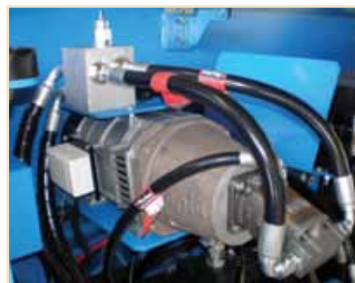
7 KVA HYDRAULIC GENERATOR
