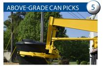
The DuraPack Rapid Rail arm can handle above-grade can picks up to 2 feet.
