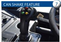
Allows the operator to shake stubborn refuse out of the container at a desired number of can shakes with a simple press of a button.
