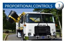
Allows for precision control while giving the operator a smoother lift and reducing cab shake.
