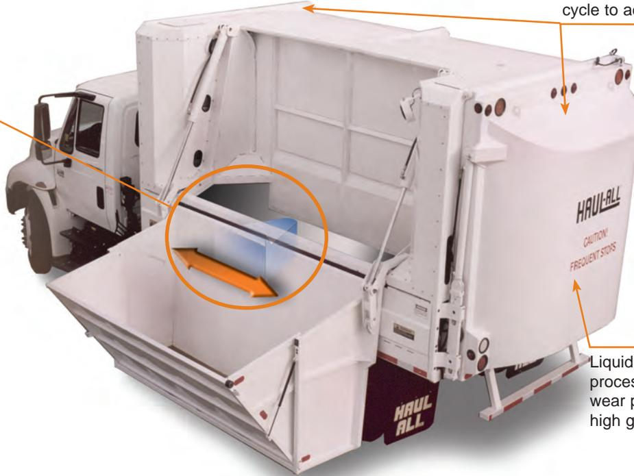
Unique panel design facilitates material flow during the compaction cycle to achieve higher payloads.
