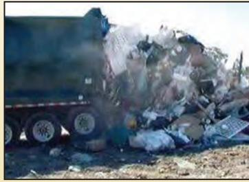
Specialized ram guides with high speed eject facilitates rapid turnaround.
