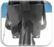
The power and coaxial cables should be run down the bike frame using wire loom, zip ties and tie mounts provided.
