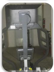
Remove the plastic boot around the neck of the machine to install the bracket and then replace with the included modified neck that has cutouts for the wires to pass through.
