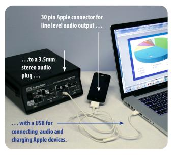
Configuration shown above utilizes an SW805 amplifier, an iPod, and a laptop computer.
