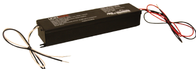
700mA 36W Hardwire Driver 120-277V AC input / Class 2 cURus / Dimmable (2-10 fixtures) LED-DR36-700D
