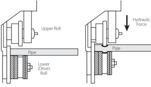
Vic-Easy tools cold form groove into pipe maintains dimensions
