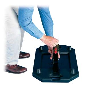
The Zephyr Portable Sign Stand is easy to use - simply release the lever and raise the mast to lock it into the upright position. No further adjustments are necessary. No folding legs that extend out into traffic.
