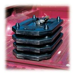
The Zephyr low profile sign stand takes up very little storage space in the truck (only 4" tall when folded). Stacking lugs are molded into the base for easy storage. The vertical mast folds down and locks in place to minimize damage during loading, transporting, and unloading the stand.
