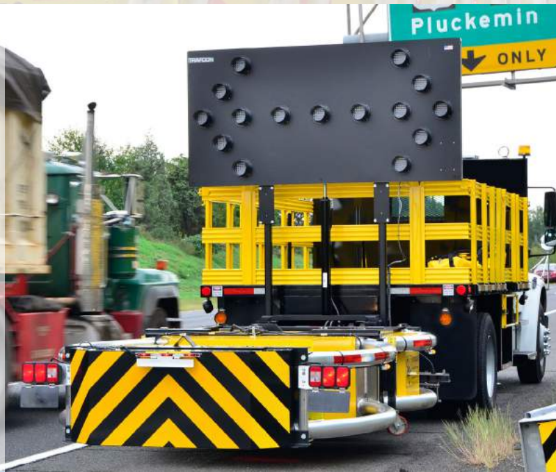
The Scorpion TMA is hydraulically powered and measures 13 feet long when fully extended, making it ideal for stationary and mobile construction zones.
