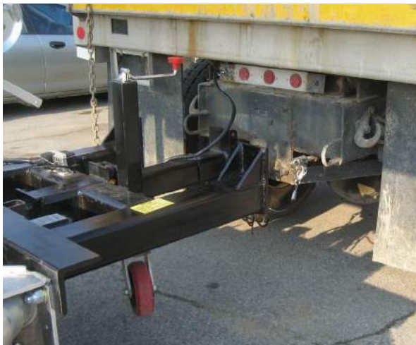
Scorpion TL-3 Trailer Attenuator with Telescoping Anti-Rotational System (TARS) allows for Single Point Attachment to Pintle Hook. The Tongue keeps the cushion positioned to attenuate "real world" angled and offset impacts efficiently without Trailer Rotation.
