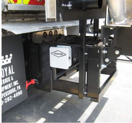
Fast-Trak w/30" Extension and Vertical Arrowboard Lift
