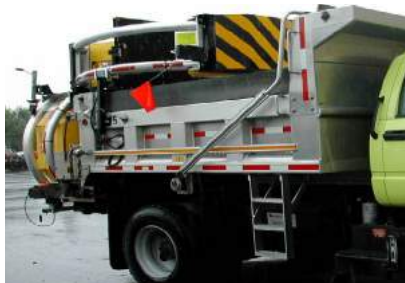
The Scorpion TMA and message panel in the storage or transport position.
