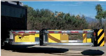
The Scorpion TMA is fully extended, with the changeable message panel in the travel or storage position.
