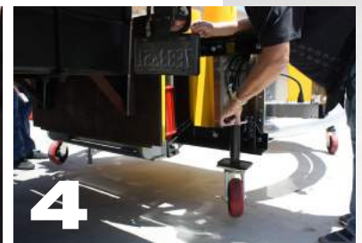
Crank jacks up and rotate for storage and insert locking pins
