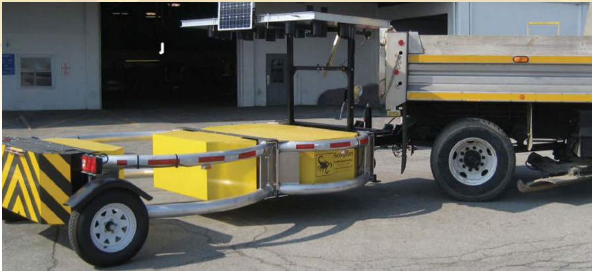
Scorpion TL-3 Trailer Attenuator with optional Arrow Board and Lift easily adapts to multiple trucks for efficient fleet management - Fast to hook up, has 45 degree turning radius, and is easy to tow and back up.
