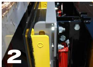
Align mounting hooks over connection bars and lower in place
