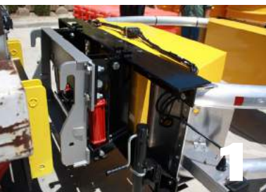
Back up truck to Fast-Trak SwiftConnect
