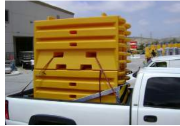
Complete SLED™ TL-3 System Transports in a Pick-Up Truck
