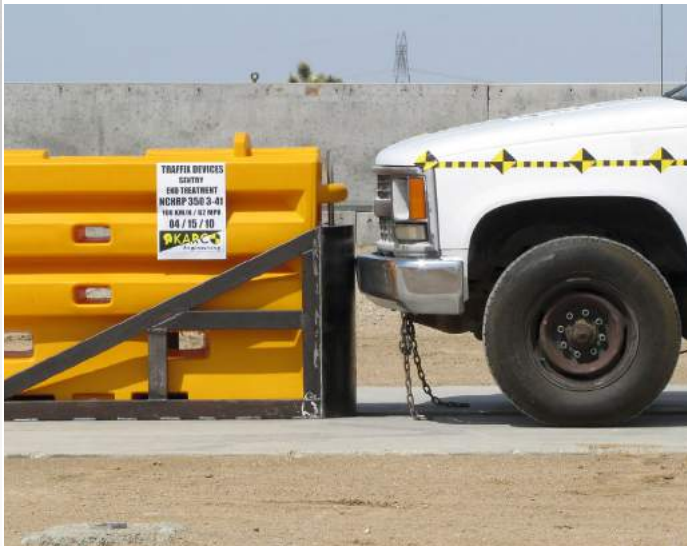
Inline TL-3 Truck Test Pre Impact
