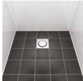
BLÜCHER® Drain Domestic SQUARE To be placed minimum 15 cm from wall
