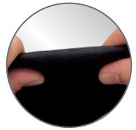
UV CHECKING: Storing in areas exposed to prolonged sunlight causes UV checking.
