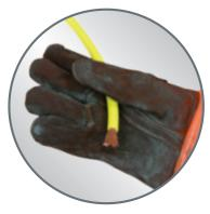
EMBEDDED WIRES: Inspect for embedded wires or metal shavings that could puncture rubber gloves.
