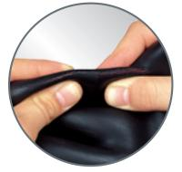
**CRACKING & CUTTING:** Shown above is damage caused by prolonged folding or compressing.
