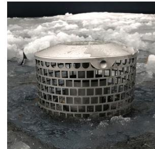
**Gravity Roof.** Stainless steel drains with a bigger opening ensure safe flow and a long service life on the roof. The large inside pipe diameter combined with the smooth stainless steel surface gives 30% higher flow capacity.
