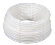
Wirsbo hePEX<sup>™</sup> features an oxygen barrier that conforms to DIN 4726 for use in closed-loop hydronic piping and radiant heating and cooling applications. The tubing is rated and listed by the Hydrostatic Stress Board of PPI at 200°F at 80psi, 180°F at 100psi and 73.4°F at 160psi. It is compatible with Uponor ProPEX and QS-style fittings and is manufactured in full compliance to ASTM F876 and F877. It is also listed to NSF 61 for potable-water applications.
