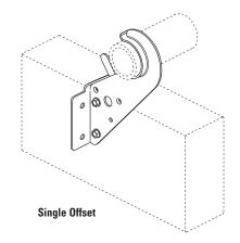
Install using a rechargeable electric drill fitted with a <sup>5</sup>/16" (7.9mm) socket attachment with the special hex head self-tapping screws provided. Install screws until they bottom out. Pipe can be "snapped" into hanger before or after installation of the screws to the mounting surface. "Thumb tab" may be bent up to provide additional protection to the pipe, but is not required for performance of the hanger / restrainer function.
