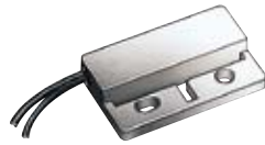
Type 4 / R4 (2) SPST Proximity 0.35 amp @ 140 VAC, 1 amp @ 50 VDC, 50 Watt Max. Minimum 1 mA
