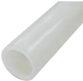
Uponor AquaPEX white tubing is marked with the PEX 5106 designation as required by the most recent edition of ASTM F876-15a, indicating it exceeds ASTM F876 chlorine-resistance requirements for continuous-recirculation systems operating up to 140°F while also affording a one-month UV-resistance level. Uponor AquaPEX white tubing ( 3/4", 1" and 1 1/4" only) is also listed to UL 1821 and ULC/ORD-C199P and carries an additional rating of 120°F at 130psi.
