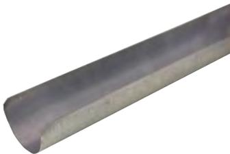
PEX-a pipe supports are made of 23-gauge, galvanized steel and are available in 1/2" to 3 1/2" sizes for suspended commercial plumbing and hydronic piping applications, enabling extended support spacing. Each package quantity contains 15 support straps (i.e., three support straps per 9-ft. length).
