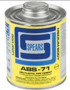
ABS-71 YELLOW/MILKY: Medium bodied, fast setting, high strength ABS solvent cement for all classes and schedules of pipe and fittings with interference fit through 8" diameter. Listings: ASTM D2235, NSF®-DWV, SW, U.P. Code, CSA (Yellow Only) B181.1.
