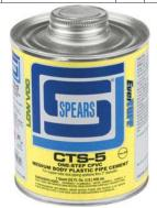
**CTS-5 EverTUFF**® **YELLOW:** Medium bodied, fast setting cement for copper tube size pipe and fittings with interference fit through 2" diameter. ONE STEP CEMENT - formulated for use without primer if local code permits. Listings: ASTM F493/D2846, NSF®-PW, DWV, SW, U.P. Code, CSA B137.6, B181.2. Maximum 2" size for One - Step use (check codes).
