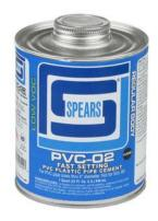
**PVC-02 CLEAR:** Regular bodied, fast setting PVC cement for all classes and schedules (except Schedule 80) with interference fit through 4" diameter. Goes on clear, dries clearest and is slightly thicker than PVC-00. Excellent for plumbing, DWV, irrigation, electrical conduit, pool & spa and PVC foam core pipe. Listings: ASTM D2564, NSF®-PW, DWV, SW, U.P. Code.
