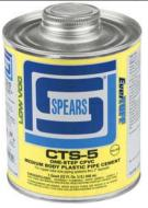
CTS-5 EverTUFF® YELLOW: Medium bodied, fast setting cement for copper tube size pipe and fittings with interference fit through 2" diameter. ONE STEP CEMENT - formulated for use without primer if local code permits. Listings: ASTM F493/D2846, NSF®-PW, DWV, SW, U.P. Code, CSA B137.6, B181.2. Maximum 2" size for One - Step use (check codes).
