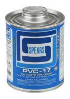
PVC-17 CLEAR/GRAY: Heavy bodied, medium setting PVC cement for all classes and schedules with interference fit through 12" diameter (non-pressure applications only up to 18"). Medium set allows more working time in warm weather and has good gap filling properties. Designed for plumbing, industrial, pool, irrigation and electrical piping systems. Listings: ASTM D2564, NSF®-PW, DWV, SW, U.P.Code (Clear/Gray); CSA B137.3, B181.2 (Gray only).
