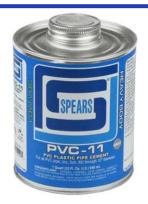
**PVC-11 GRAY:** Heavy bodied, medium setting PVC cement for all classes and schedules with interference fit through 12" diameter. Medium set allows more working time in warm weather and has good gap filling properties. Listings: ASTM D2564, NSF®-PW, DWV, SW, U.P. Code, CSA B137.3, B181.2.
