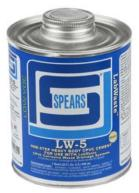
**LW-5 MUSTARD:** One-Step (no primer required) CPVC cement specifically formulated and approved for use with Spears® **LabWaste**® CPVC Corrosive Waste Drainage System Products with interference fit through 24". See Publication LW-4, Technical Information, for application details. Listings: ASTM F493, NSF®-CW, PW, DWV, SW, U.P. Code, ICC-ES PMG. **For use in joining LabWaste® only**.
