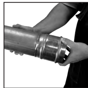
Figure 9: Inspection of final crimp
