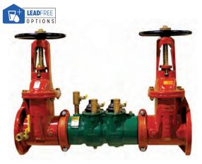
The Apollo<sup>®</sup> DC 4SGLF /4SG / 4S Series Double Check Valve is designed to prevent contamination of the potable water supply due to back-siphonage or backpressure from substances that are non-health hazards. The modular check valves have replaceable seats and reversible EPDM seat discs. Grooved connections on an epoxy-coated ductile iron body allow for easy connection to butterfly valves or gate valves (2-1/2" - 8"), flanged (10" only).
